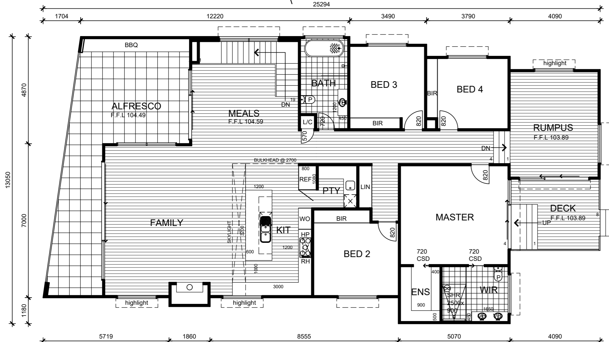
GROUND FLOOR PLAN Proposed Scale 1:100
