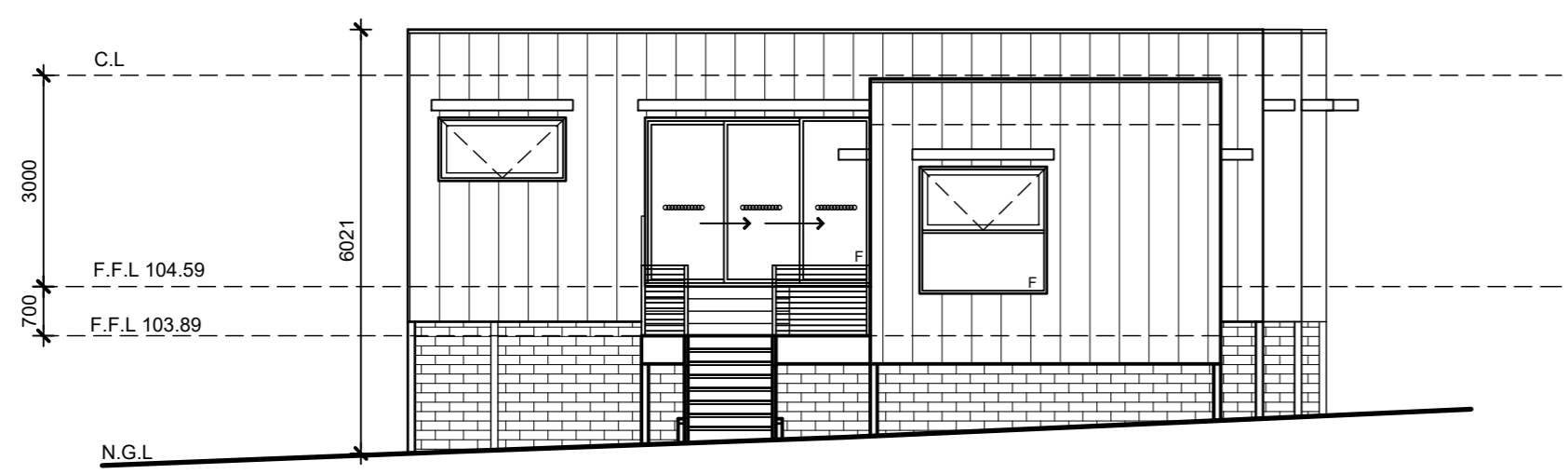
SOUTH EAST ELEVATION Scale 1:100
